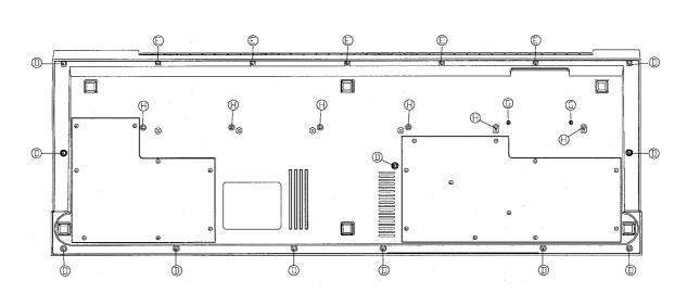
Turn the keyboard over again and fold up the complete front panel. The **"Main Board"** (main control board) of the *iS40/iS50* will become visible.
