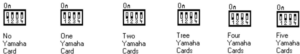
Put the switches in the right positions like the picture above demonstrates.
